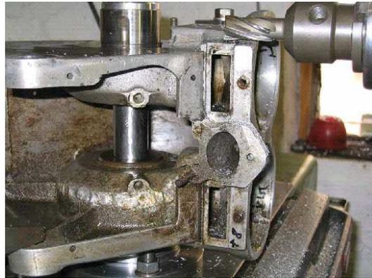
The crankcase can now be carefully clamped and then the barrel seating face skimmed to restore flatness and truth to the main bearings. Whilst in this position, two small location faces are machined on the section that the transfer port cover bridges over each side. We now have a seating face and axis alignment faces for any further operations.
