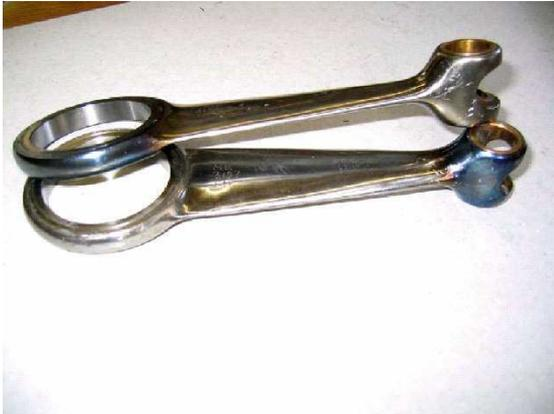
Consequences of little end alignment faults. Alignment should be within 0.001" measured both sides of the rod little end, in two axis to check both parallelism and twist. Rod with "blue" little end measured
