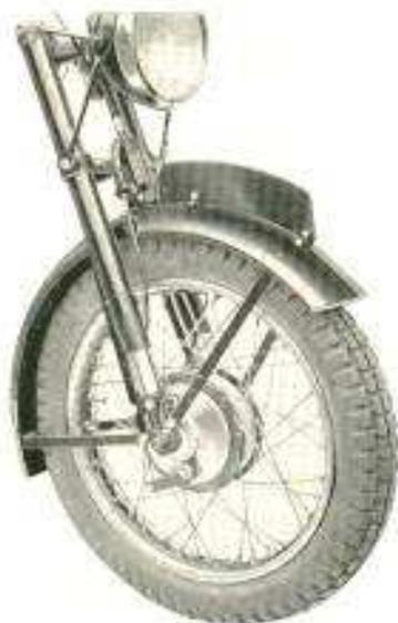
**FRONT FORK.**—Scott-Dowty "Oleomatic" Telescopic, giving six inches of progressive air springing with constant oil damping. Individual adjustment for any riding condition—solo, pillion or side-car. Adjustable friction type steering damper. The fork can be assembled immediately in the frame of any Flyer-Tourer or Replica Model, which is at present fitted with ball races in the steering head. Frames fitted with taper roller bearings require special adaptor rings. Type must be stated.
